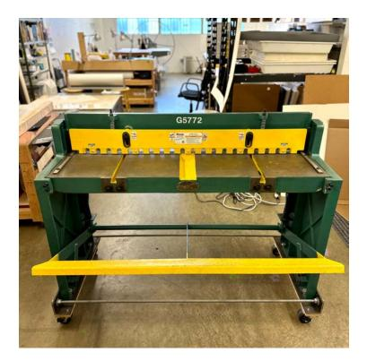
Light surface rust in some areas of the bed (raw steel). Used occasionally by one person to cut copper plates 18-20 gauge. Includes front and rear extensions arms, rear adjustments blocks and bevel gauge. The shear is on skates with locking casters for ease of transportation. The shear is to be taken off the skates before use.
